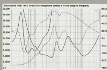
Fig.2 mbl 101E, individual electrical impedance (solid) and phase (dashed) of upper-frequency and bandpass woofer sections (2 ohms/vertical div.)
