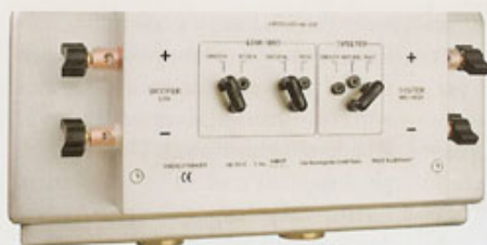
A small jumper is used to fine-adjust the 101E to the listener's environment and sound preferences.
